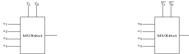
FIGURE 4 – \text{MUX4to1}(a_4 a_3 a_2 a_1, T_1 T_0) et \text{MUX4to1}(a_3 a_2 a_1 a_0, \overline{T_1} \overline{T_0})
